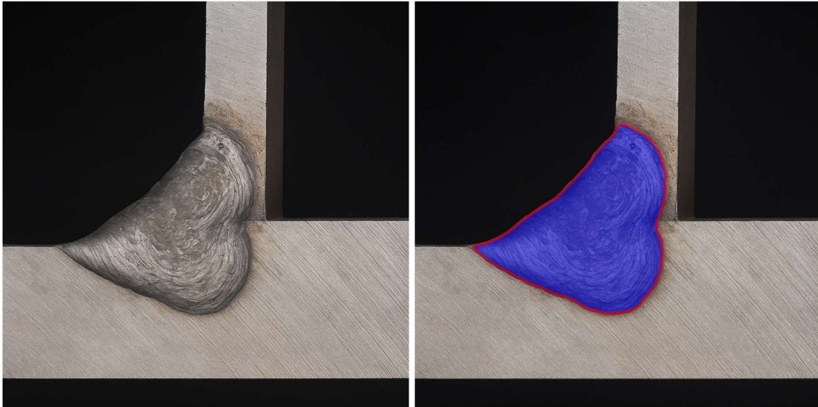
Figure 2. Original weld image and corresponding automated segmentation of the region of interest using image analysis.
