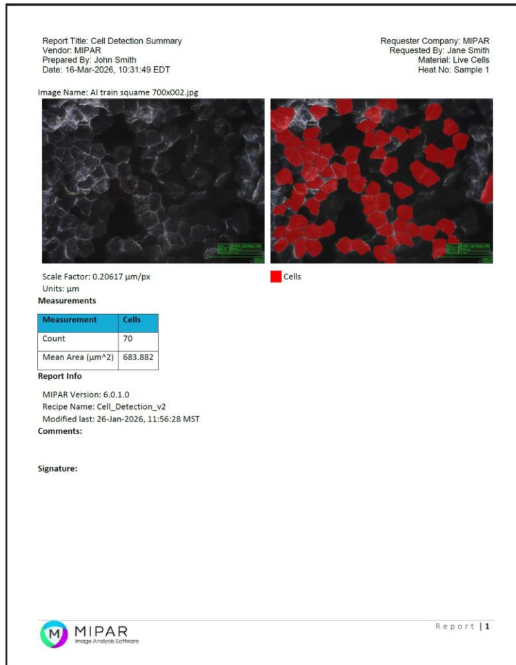
Figure 5. MIPAR Summary Report showing raw image and detection overlay side by side, spatial calibration (scale factor and units), aggregate measurements (cell count and mean area), recipe version, and fields for comments and signature to support traceability requirements.
